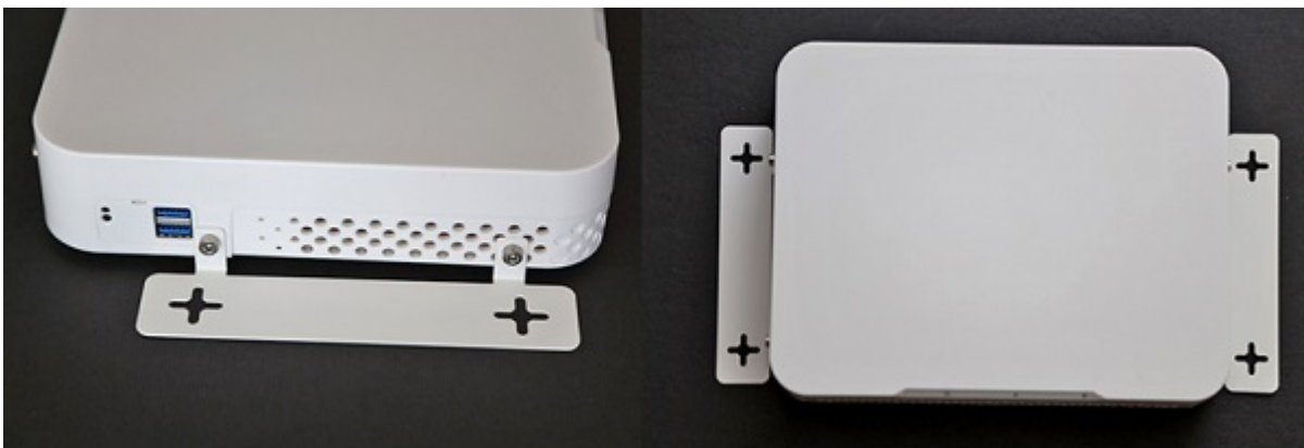
Fig. 19: The Netgate 8200 Outboard Wall Mount Orientation
