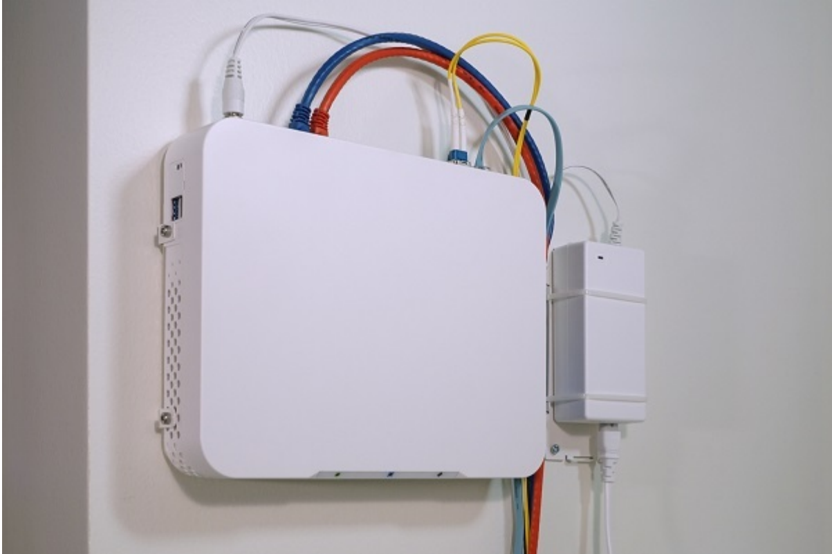
Fig. 16: The Netgate 8200 Mounted Vertically
