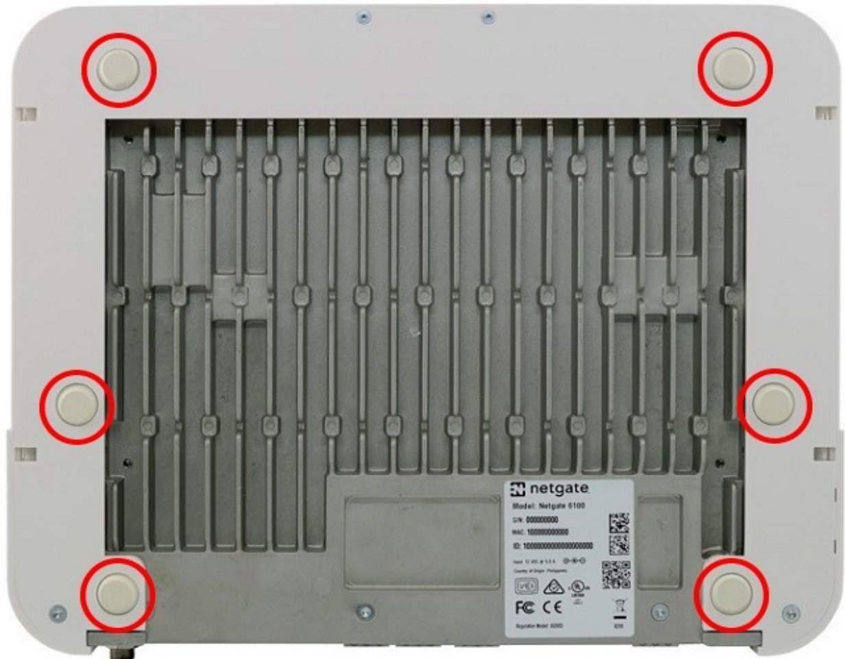
Fig. 6: Remove the Rubber Feet
