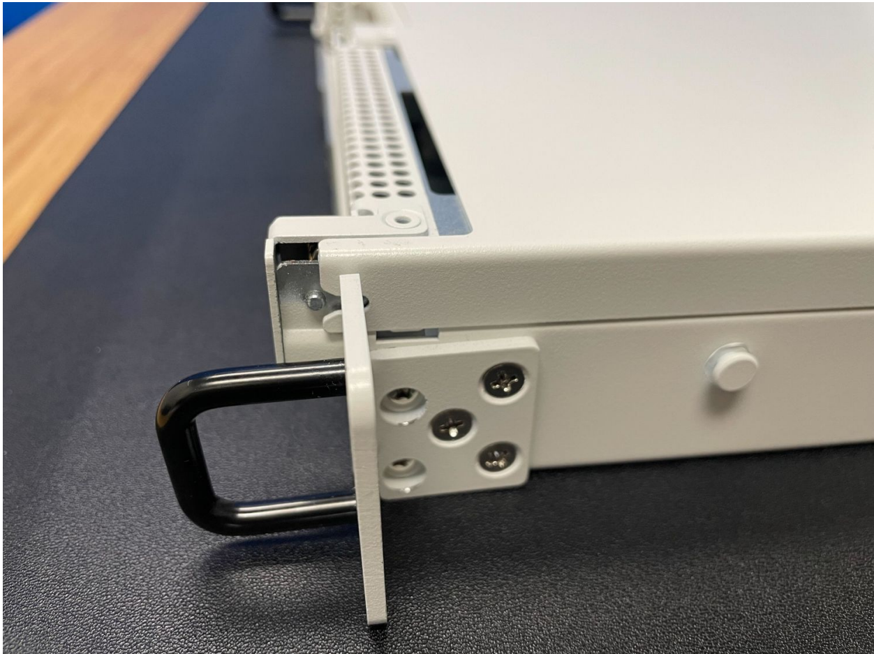
Fig. 29: Slide the top cover back toward the front panel
