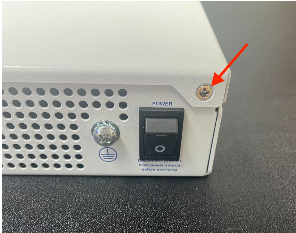
Fig. 84: Screw on the rear side of the unit at the right top corner, indicated with an arrow.
