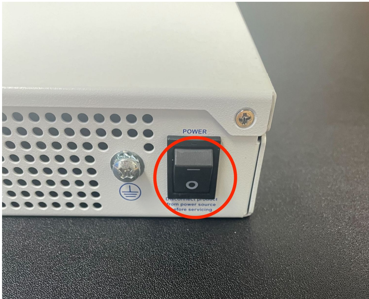
Fig. 34: Power switch (circled) in the off position
