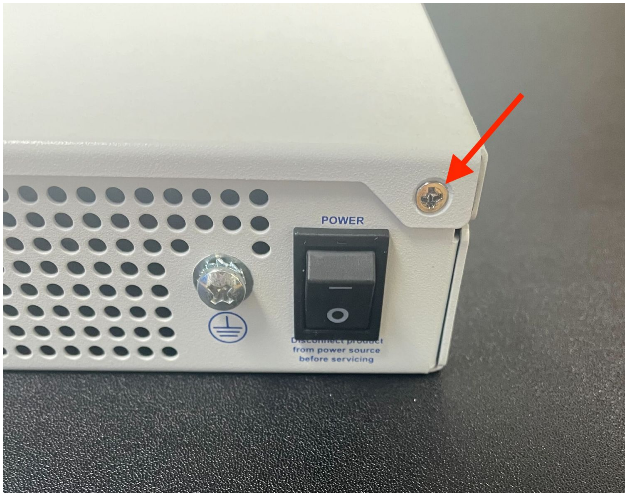
Fig. 61: Screw on the rear side of the unit at the right top corner, indicated with an arrow.
