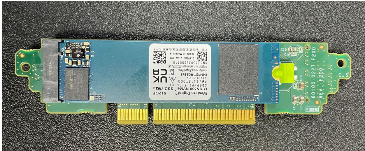
Fig. 47: M.2 NVMe riser card slot 2 with the add-on SSD installed
